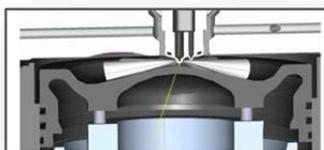
Combustion shape in combination with fuel injection & use of higher max. cyl. pressure
