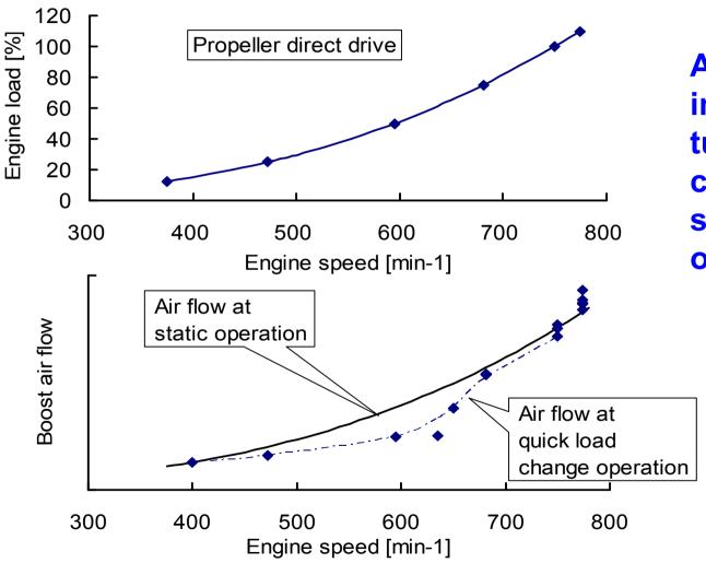
At quick load increase, turbocharger cannot supply a sufficient amount of air.
