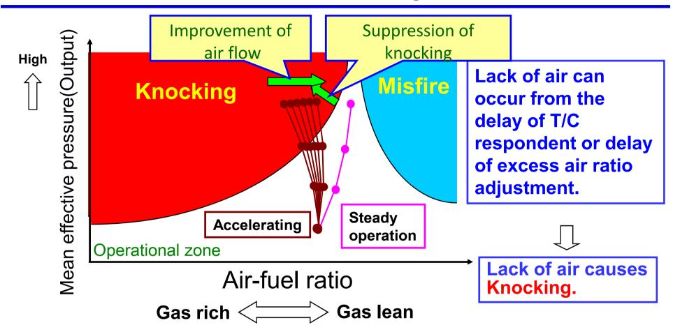
To improve transient performance, secure of sufficient air flow and suppression of knocking is necessary
