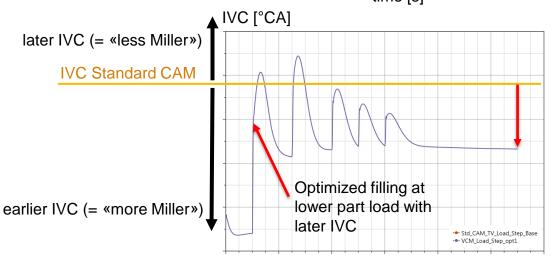
Full load: earlier IVC to gain engine efficiency & enabling increased cylinder compression ratio
