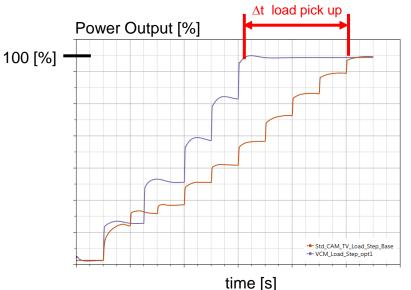
Calculated for high-speed gas engine, port injection & 2-stage turbocharging
