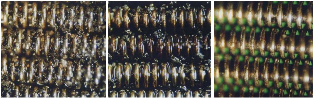
Figure 2: Left: Asphaltenes and cat-fines retained on the upstream side of a 25 micron mesh Middle: More asphaltenes on the downstream side of this 25 micron mesh Right: The same mesh after washing with distillate fuel
