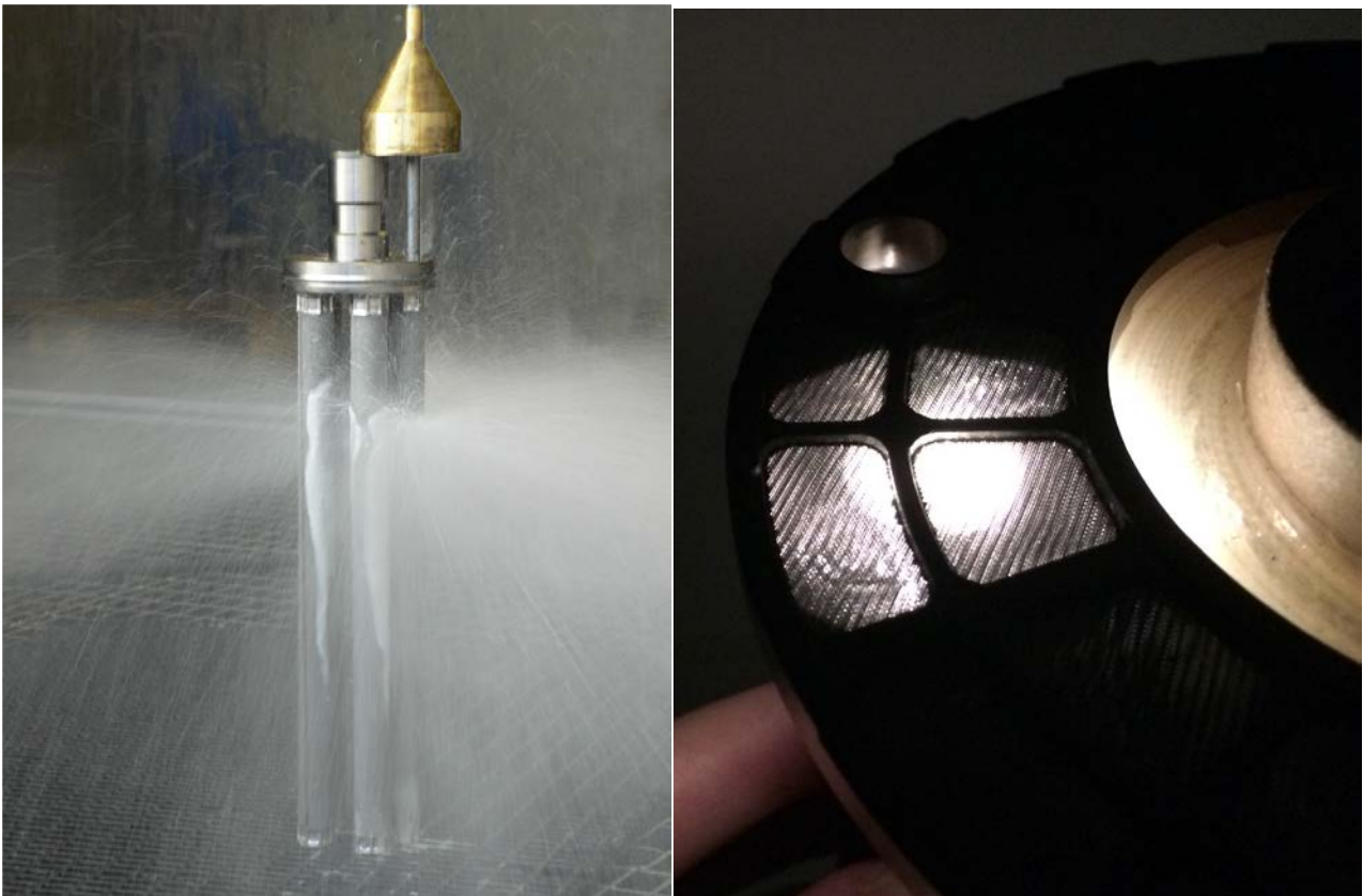
Figure 4: Clean mesh allows the ready passage of water (left); and light, seen here against a disc element (right)
