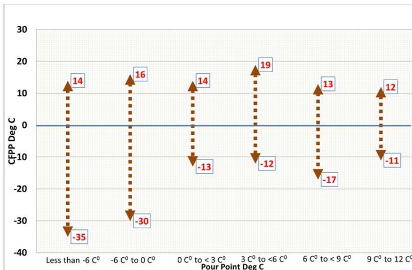
Figure 3: Max / Min CFPP range for DMA grade distillates against Pour Point - Global coverage 2013/14 (Courtesy of LR FOBAS)
