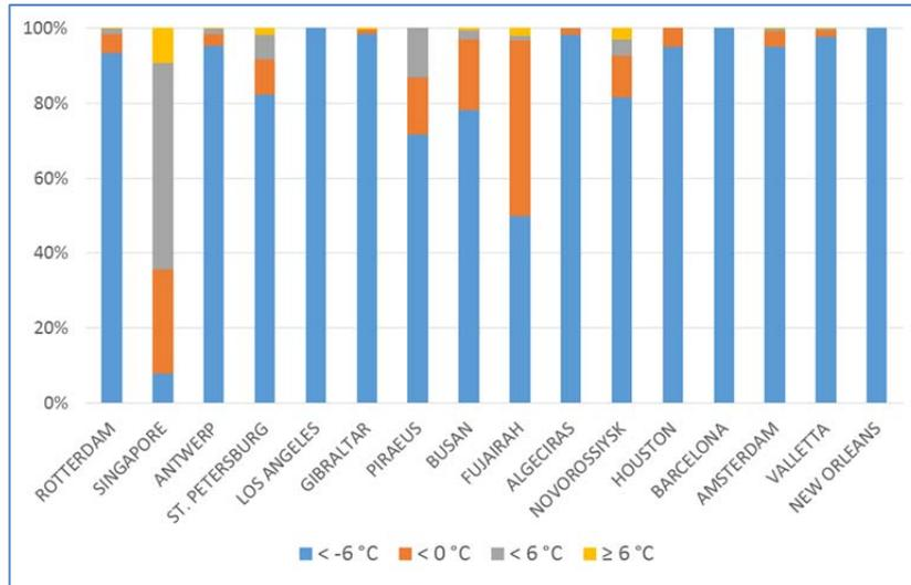
Figure 2: Distribution of pour point in DMA grade distillates in some main ports, Aug 2013 - Aug 2014 (Courtesy of VPS)
