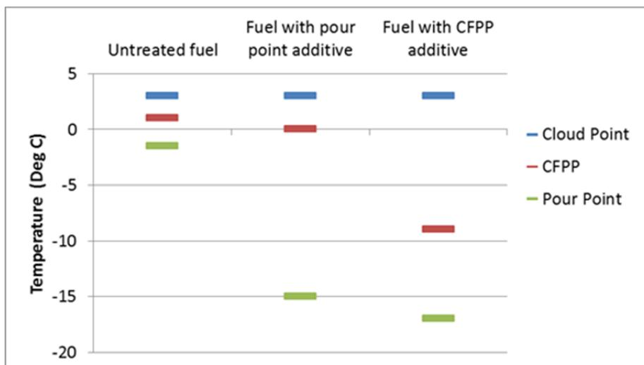
Figure 5: The impact of different additives on reducing the CFPP and PP (courtesy of Infineum)
