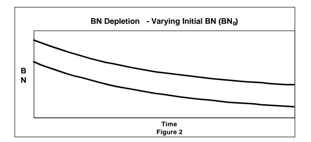
Increase of the initial BN has a purely linear effect and may raise the stable state to above that of the engine builders limit. An alternative approach is to renew the sump charge and the economic consequences of this are considered in a later section.
