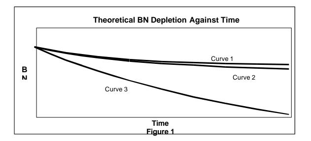
All engine builders have a limit for alkalinity depletion, that is sometimes expressed as a percentage of the initial BN, or as a numerical value. If this limit is approached in service, corrective action has to be taken. One approach is to use an oil with a higher initial BN. The effect of this is shown in Figure 2.
