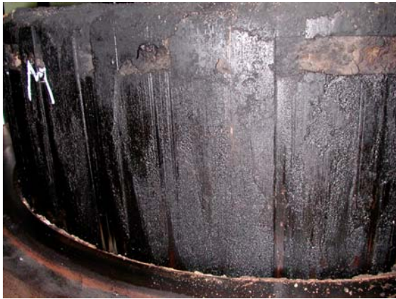
Fig 2: CaCO 3 Deposits on piston top
