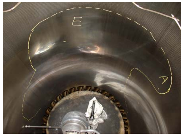
Fig 3: Bore polish of liner
