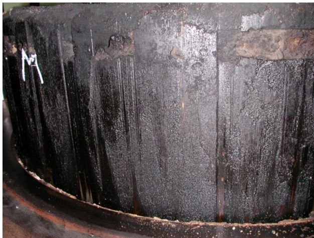
Figure 20: Excessive top land deposits
