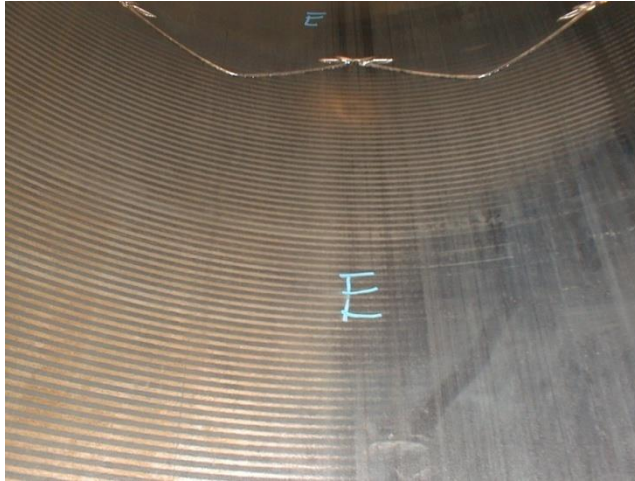
Figure A16: Example of bore polishing
