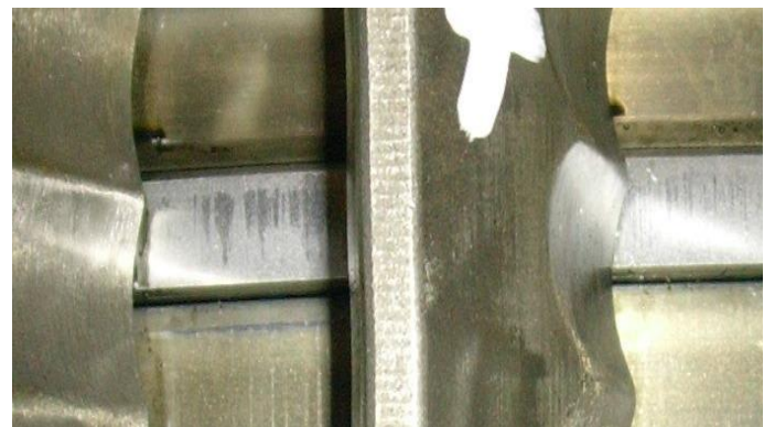
Example: Micro seizures of the piston ring
