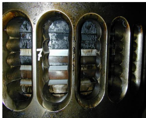
Example: Broken piston ring
