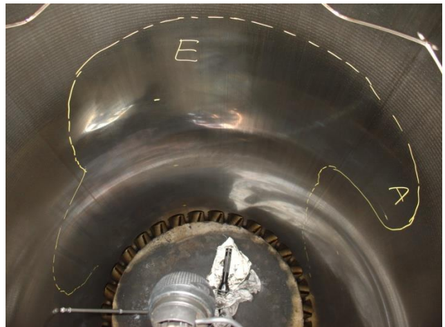
Figure 21: Bore polish of the cylinder liner by excessive top land deposits
