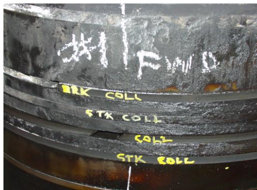
Figure 17: Poor piston cleanliness caused by lubricant chemistry – broken, stuck & collapsed piston rings
