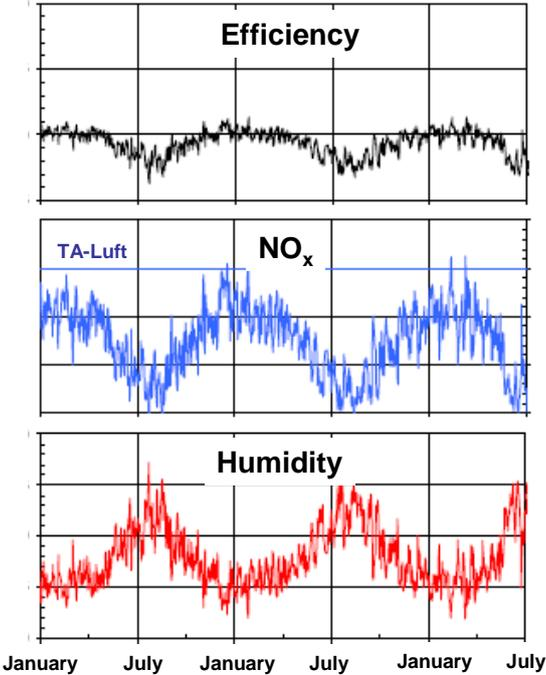
Another effect of high humidity is the possible condensation of water in the charge air cooler if the temperature drops below the dew point temperature at the given pressure. Without drain, this can have harmful effects on the engine operation and must be avoided.
