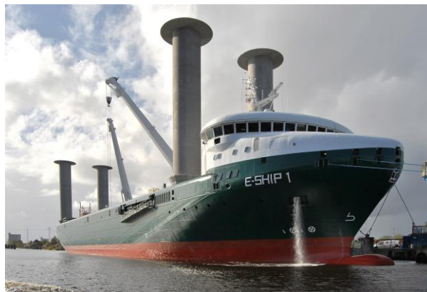
Figure 8: Example of a wind assisted propulsion technology [Die E-Ship 1 im Emden Hafen]
