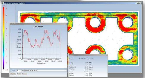
Design 2:  $A_c = 7888 \text{ mm}^2$   $A_p = 11439 \text{ mm}^2$  $\sigma_v = 40 \text{ MPa}$
