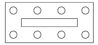
Design 1:  $A_d = 17000 \text{ mm}^2$  $\sigma_v = 18 \text{ MPa}$
