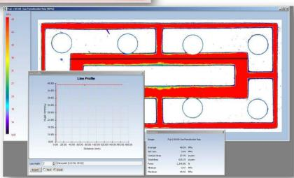
Design 3:  $A_c = 7878 \text{ mm}^2$   $A_p = 2520 \text{ mm}^2$  $\sigma_v = 40 \text{ MPa}$
