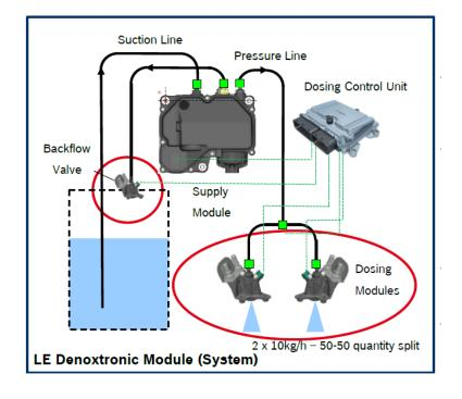
Automotive base DENOX-LE system is reliable SCR system covering 1MW...5MW engines.
