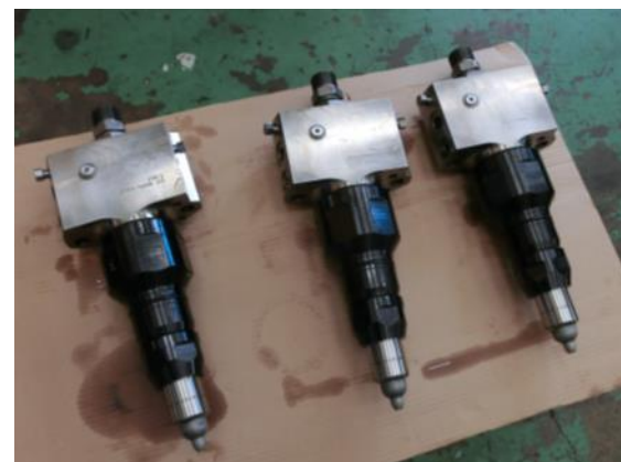
Fuel injection valve(with water injection line)
