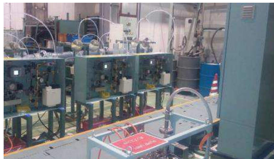
Shop test of Urea dosing system at Amagasaki factory
