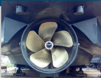
Inland water ways Propeller diameters < ~3 m
