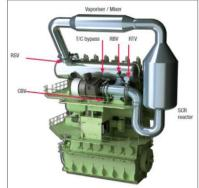
\* RSV : Reactor Sealing Valve, RTV : Reactor Throttle Valve, RBV : Reactor Bypass Valve, CBV : Cylinder Bypass Valve, TBV : T/C Bypass Valve
