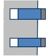
Piston ring grooves with thick chromium layer
