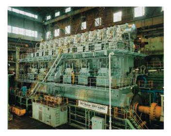
Fig. 110 The first 12-cylinder Sulzer RTA96C engine on test at Diesel United in Aioi, Japan. (Wärtsilä)
