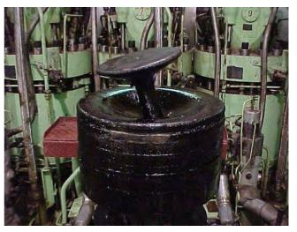
Fig. 116 Broken valve spindle forged through piston crown. (Author)
