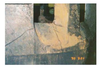
Fig. 97 Cracked cylinder liner, KSZ90BL. (Author)
