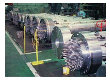
Fig. 113 Cooling inserts for pistons, RTA96C. (Wärtsilä [74])
