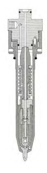
Fig. 55 Slim Fuel Valve for all B&W 2-stroke engines (B&W)
