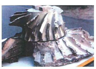
Fig. 99 Blower wheel of complete wrecked turbocharger (Author)
