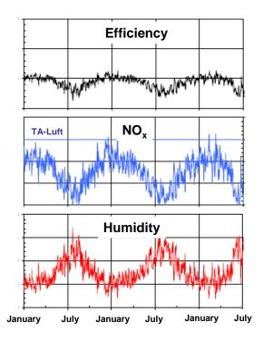
Another effect of high humidity is the possible condensation of water in the charge air cooler if the temperature drops below the dew point temperature at the given pressure. Without drain, this can have harmful effects on the engine operation and must be avoided.
