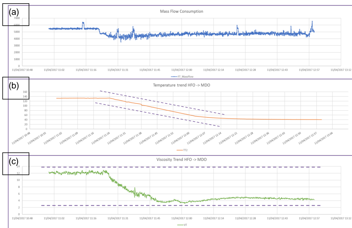
Figure 36 - Fuel changeover diagram from HSFO to distillate fuel (Alfa Laval)
