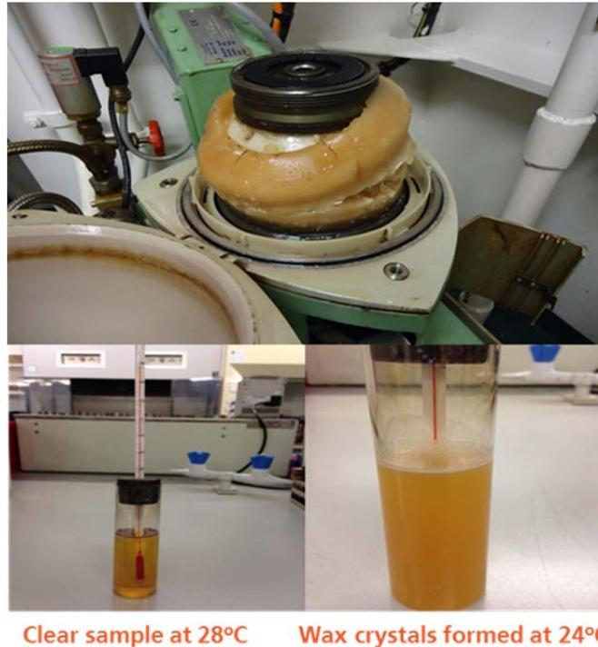
*Figure 4: Wax deposition in the diesel purifier where the distillate fuel temperature is below the CFPP of the fuel*
