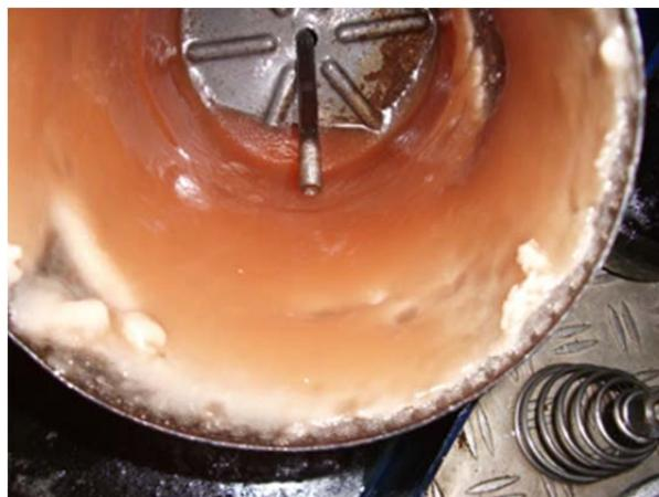
*Figure 1: Filter blocked due to wax deposit*
