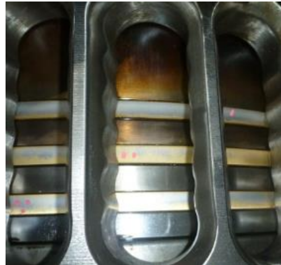
Figure 14.2: Continuous operation on gas and 100 BN cylinder oil keep the engine clean in the ring belt and might contribute to adverse build-up of exhaust system deposits.
