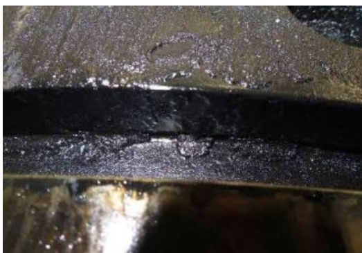
Figure 14.5: Deposits on top ring groove.
