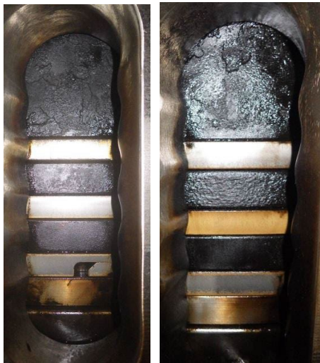
Figure 14.1: Continuous operation on gas and low-BN cylinder oil leads to ring land deposits and deposits behind the piston rings.
