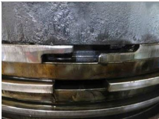
Figure 14.3: Operation on gas and low-BN leads to ring land deposits.
