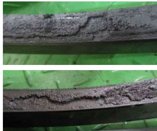
Figure 14.4: Deposits on top ring backside.
